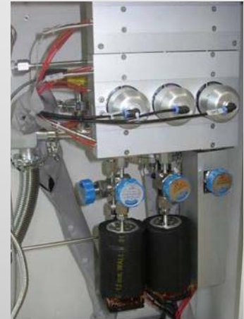
Compact source delivery system in Lucida D100 ALD
