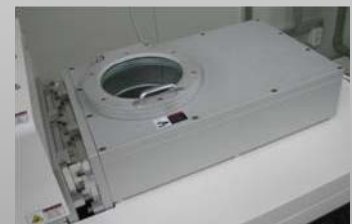
Load lock with Automatic transfer system
