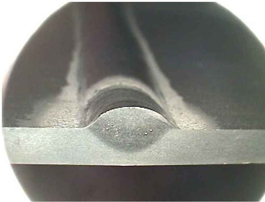
ac-TIG welding (with filler metal)
